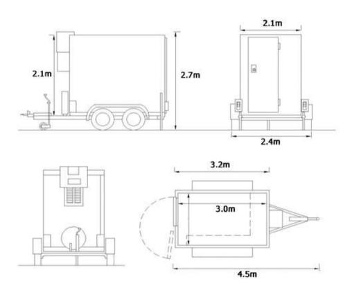
Capacity: 10.8 m<sup>3</sup> Gross Weight: 3.500 kg Pay Load: 2.400 kg
